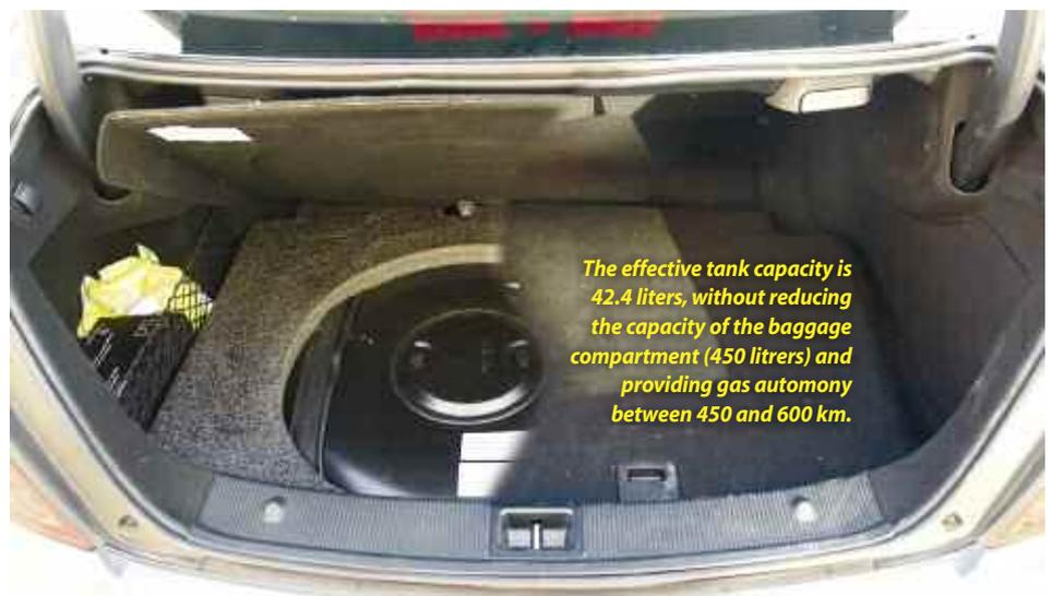
*The effective tank capacity is 42.4 liters, without reducing the capacity of the baggage compartment (450 liters) and providing gas autonomy between 450 and 600 km.*
